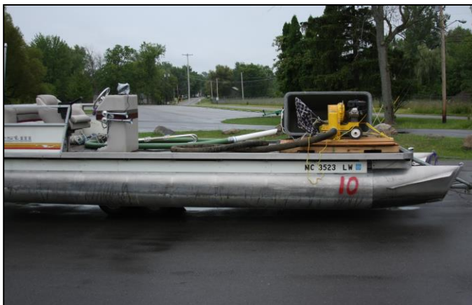
Figure 23. A DASH boat for hand-removal of milfoil or other nuisance vegetation. ©Restorative Lake Sciences, LLC
